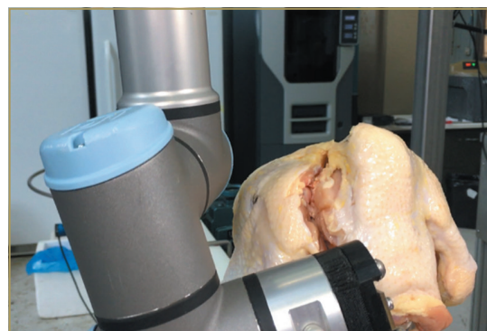
Figure 2. The learned deboning strategy was deployed on a 6 degrees of freedom robot manipulator, and the manipulator was able to perform a cut with a much more natural and smoother motion compared to the motion programmed by engineers.
