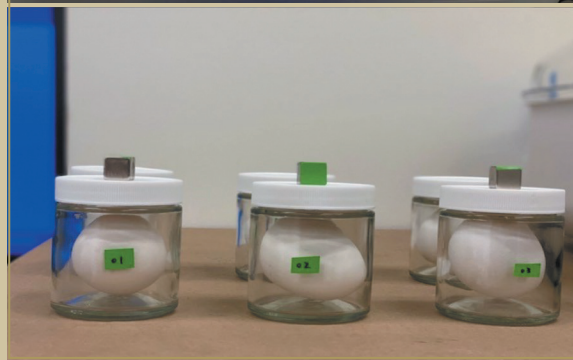
Incubator and setup for collecting volatile organic compounds (VOCs) from eggs.
